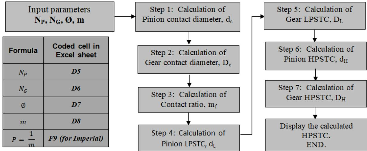
Fig. 4. Methodology for HPSTC calculation
