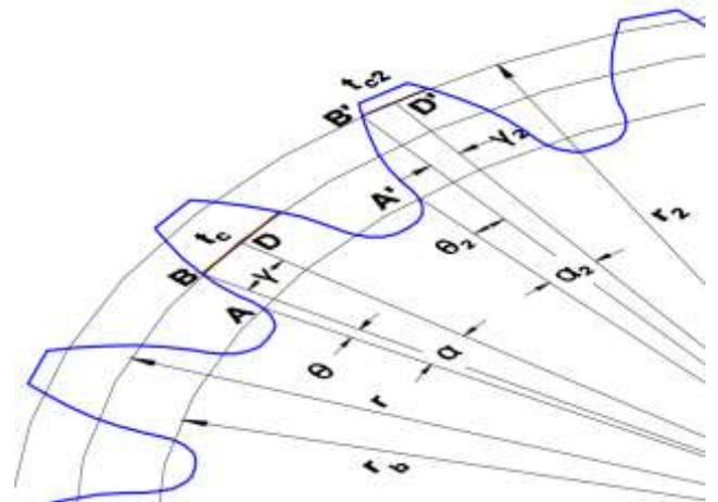
Fig. 2. Tooth thickness calculation
