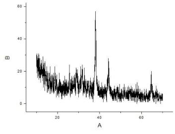
Fig. 4. XRD pattern of gold nanobiocomposite of asparaginase
