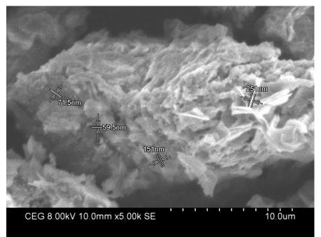
Fig. 5. SEM image of gold nanobiocomposite of asparaginase
