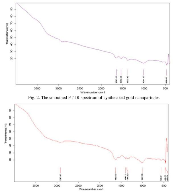
Fig. 3. The smoothed FT-IR spectrum of gold nanobiocomposite of asparaginase
