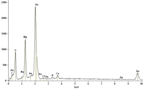
Fig. 6. EDX pattern of gold nanobiocomposite of asparaginase
