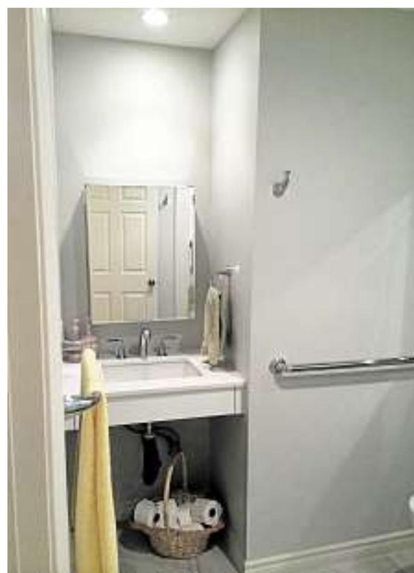
A floating vanity 29" from the floor to the underside of the unit allows the arms of the wheelchair to comfortably fit under.
