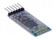
Bluetooth is a wireless technology standard for exchanging data over short distances using short-wavelength UHF radio waves in the ISM from 2.4to 2.485 GHz from fixed and mobile devices, and building personal area networks. The first channel starts at 2402 MHz and continues up to 2480MHz in 1MHz steps. It usually performs 1600 hops per second, with Adaptive Frequency-Hopping (AFH) enabled.
