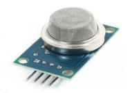
The MQ 135 Quality Detector Sensor Module For Arduino has lower conductivity .When the target combustible gas exists, the conductivity of the sensor is higher along with the gas concentration rising. The MQ 135 sensor has high sensitivity to Ammonia, Sulphide and Benzene steam, also sensitive to smoke and other harmful gases
