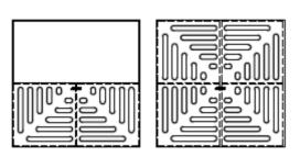
**Engineering Specification:** Construction 304 Stainless Steel Body Fully Welded; Variety of Drainage Covers; Optional Sediment Basket. Meets The ASME A112.6.3 requirements.
