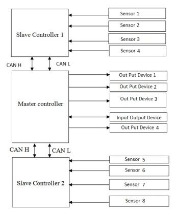
Fig 2: "System level block Diagram of vehicle control"
