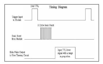
Fig 4: "Tx and Rx wave form of HC-Hr 04"
