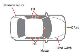
Fig 1: Vehicle with sensor network
