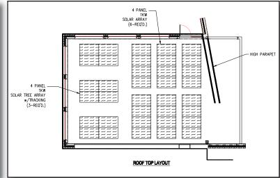
Each student station will be attached to a 1KW solar array. Six of the stations will be static arrays on the roof. Three of the stations will be "Trees" that allow sun tracking.
