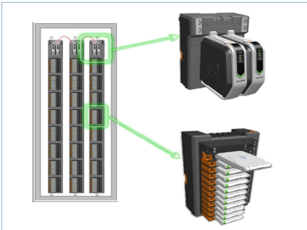
Delta-V Electronic Marshalling with CHARMS Modules and CHARMS IO Cards
