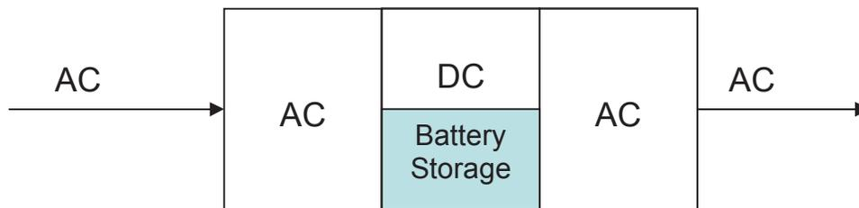
Fig 3: Present UPS usage with AC source
