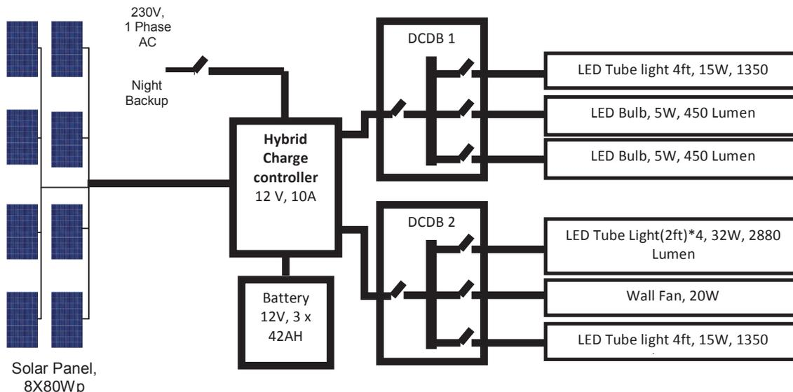
Fig 6: NETRA's DC Microgrid
