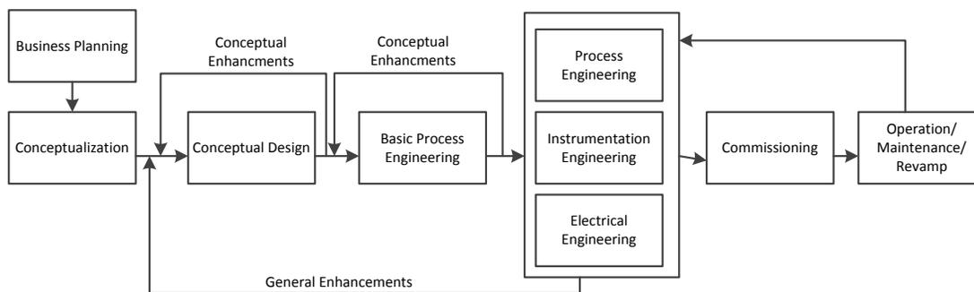
Figure 1 Traditional Sequential Process and Plant Design
