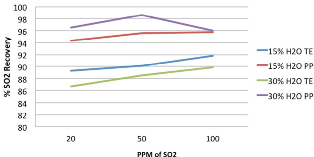
Figure 4: SO<sub>2</sub> Recovery in Cooler Vs Nafion
