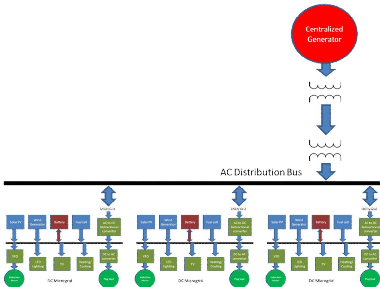
Fig : 5 DC Microgrid in interconnection with AC utility grid
