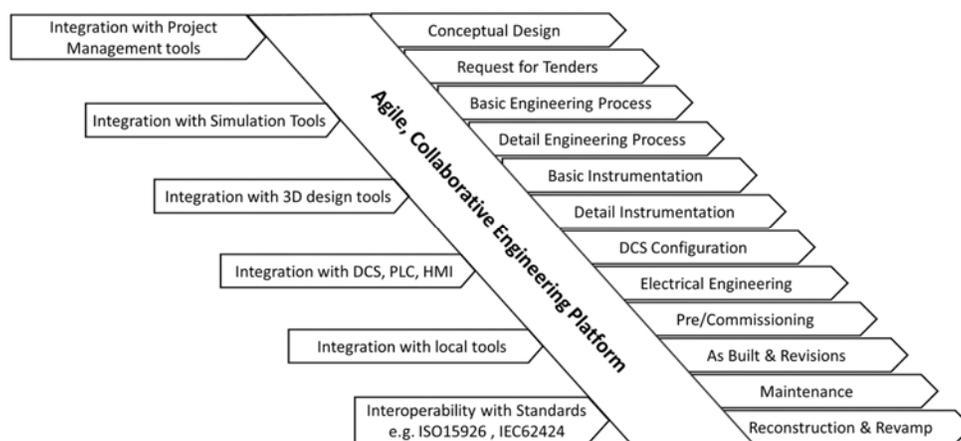
Figure 2 Collaborative Modern workflow for Plant Design
