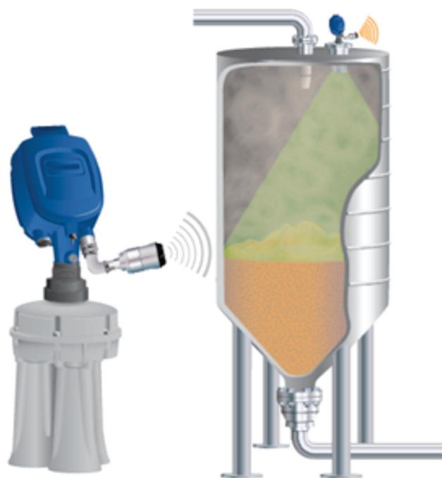
Rosemount non-contacting 3D Solids Scanner which measures average, minimum and maximum levels, and provides 3D visualization of stored contents. Using dust penetrating low frequency acoustics waves to generate surface mapping of stored materials, the 3D Solids Scanner takes the guesswork out of solids level measurement.
