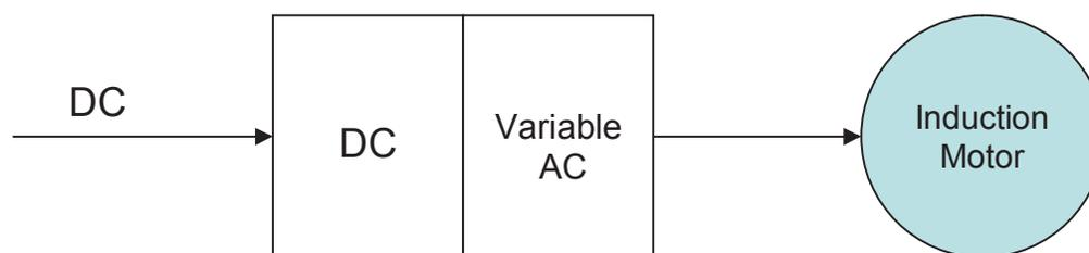
Fig: 2 Proposed VFD usage with DC source
