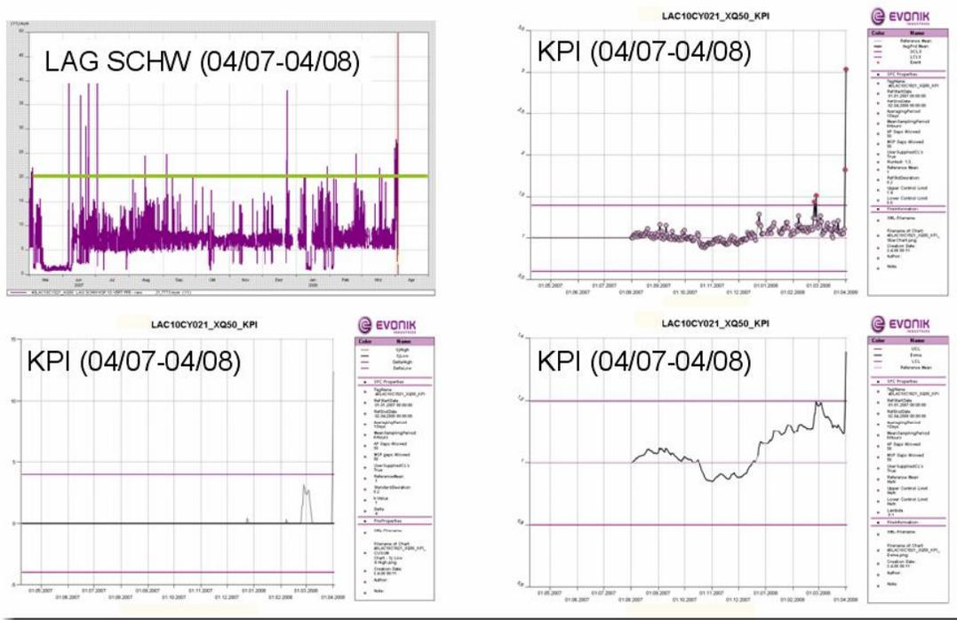
Fig. 4: Incipient crack of the shaft of a boiler feed pump → increased bearing vibrations
