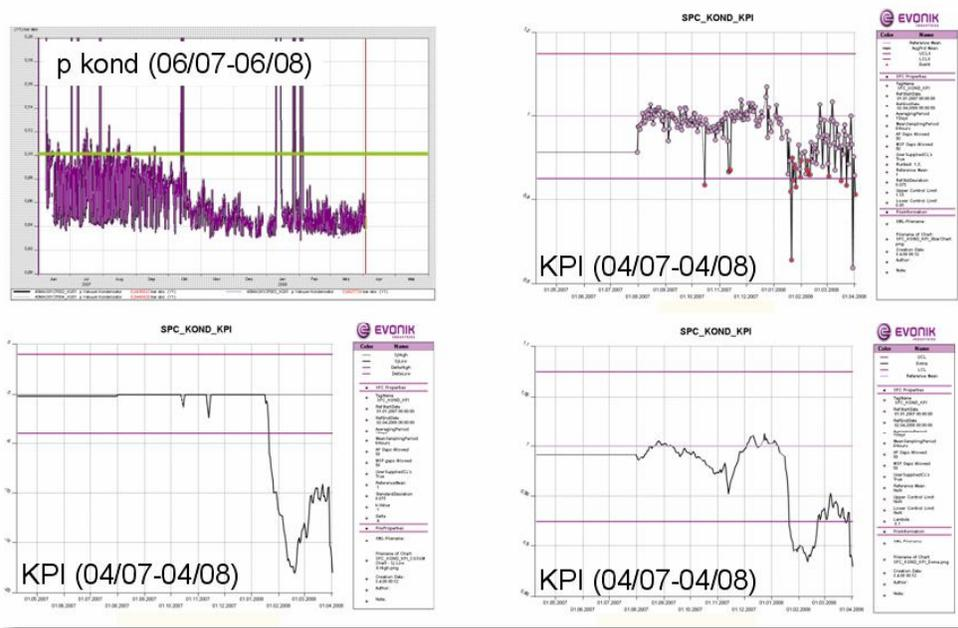
Fig. 3: Decline of process quality: condenser in off-design operation
