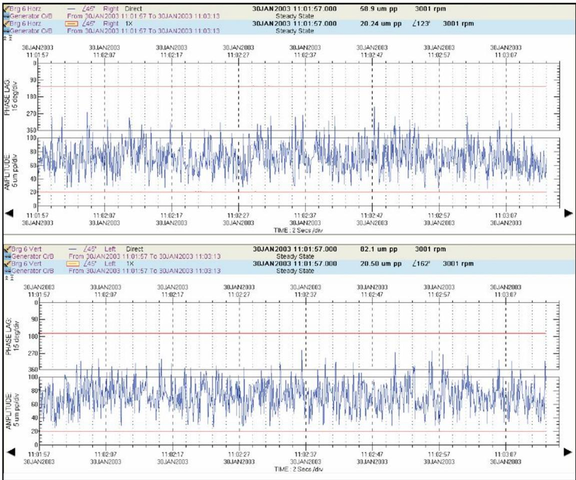
**Figure 2 – Direct and 1X vibration trends on bearing 6 showing erratic behavior (top plot shows X probe, bottom plot shows Y probe).**
