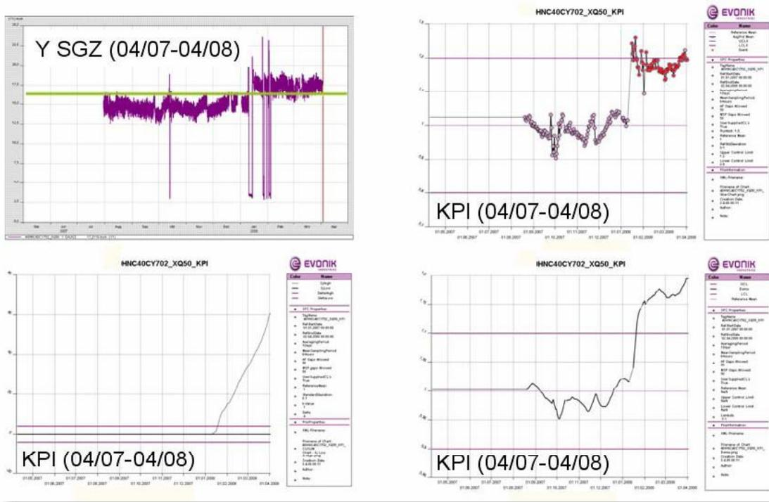
Fig. 5: Fouling on the blade of an ID fan → increased vibrations
