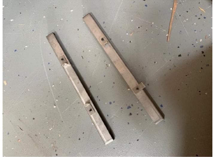
10. Either way you remove burner you now need to make sure the brackets that hold burner are back in place so you can replace with new burner. Then it best to install new burner through front hole of roaster and attach screws on the front side of burner:
