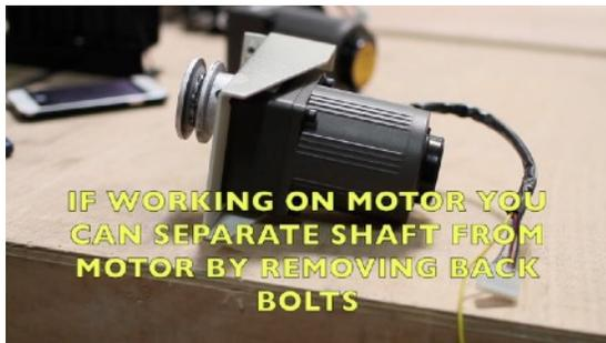
TO REMOVE DRUM MOTOR: Remove the 4 bolts in back of roaster: Then rather than remove wiring you can just set drum motor on blocks of wood beside roaster
