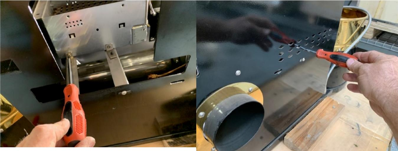
6. If the above method works for you then you will need to remove the electrical wiring from burner and to igniter needle before you can remove the burner. A #10 metric wrench and a hex key will aid in doing this. Also you will need a screwdriver to remove the black ground wire:
