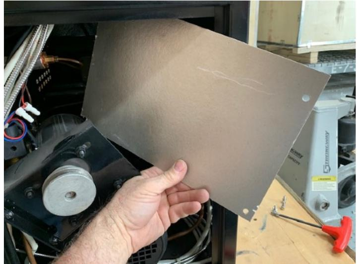
4. At this point you can do part of the work from back utility door as well as front if you remove front panel. If you prefer to do all work from back utility door you will likely need to remove the entire burner and braces holding burner onto roaster. Before doing that you need to disconnect the gas line from burner using a #12 metric wrench and gently turning counter clockwise:
