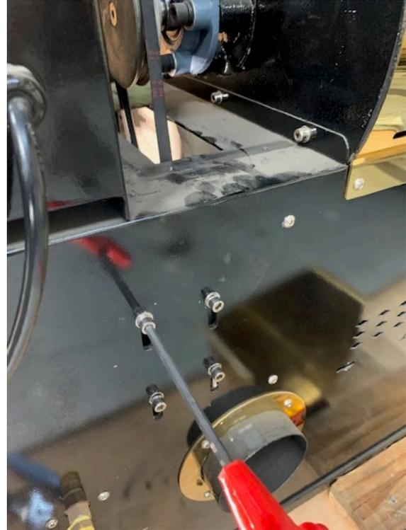
16. Test roaster: Test that drum motor is not vibrating which could indicate the belt is not tight or motor is slightly out of alignment. If it is readjust.
