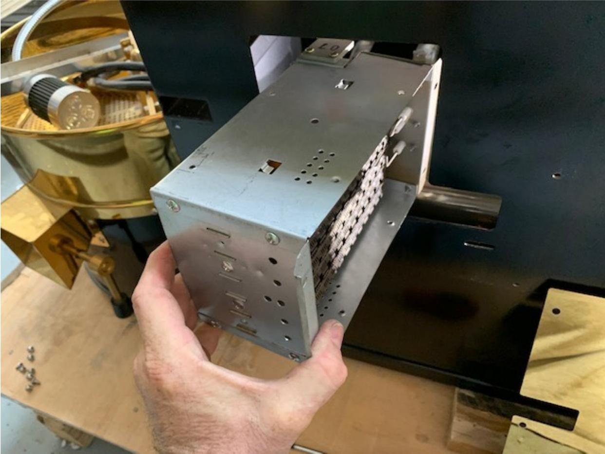
8. If you find that method too difficult you can always remove burner from back utility door. If removing from back door you may need to remove the back braces that hold up the burner if you are unable to remove the 4 screws holding it to braces as shown above. To remove burner and its braces you will see two hex bolts on front and back of roaster as seen below:
