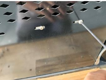
9. But if you remove the brackets holding burner to roaster you will likely need to then remove the brackets from burner before you can get all out of roaster. Generally if you can remove burner from front of raster and leave the brackets in place this will save much time and be easier:
