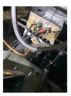
5. At this point you can either remove burner while keeping the braces below it in place by opening up front panel and unscrewing the two screws on the front side (then unscrewing the back side by putting a long Phillips driver through vent holes in back:)
