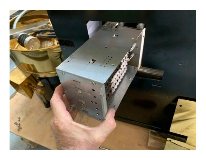
8. If you find that method to difficult you can always remove burner from bak utility door. If removing from back door you may need to remove the back braces that hold up the burner if you are unable to remove the 4 screws holding it to braces as shown above. To remove burner and its braces you will see two hex bolts on front and back of roaster as seen below:
