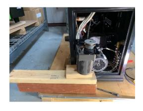
3. Next remove firewall: 4 small hex bolts hold firewall on inside of roaster
