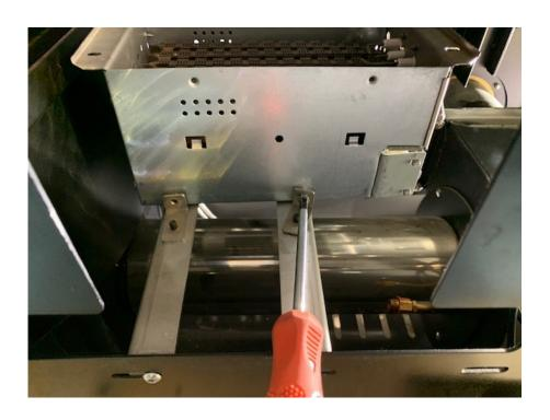
11. Then to attach the screws to back side of burner you may be able to do this from the inside of roaster with a small screwdriver or using a bit of tape on the end of a long screwdriver you can put screws on the same way you removed them:
