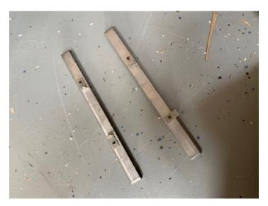
10. Either way you remove burner you now need to make sure the brackets that hold burner are back in place so you can replace with new burner. Then it best to install new burner through front hole of roaster and attach screws on the front side of burner:
