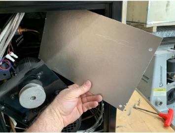
4. At this point you can do part of the work from back utility door as well as front if you remove front panel. If you prefer to do all work from back utility door you will likely need to remove the entire burner and braces holding burner onto roaster. Before doing that you need to disconnect the gas line from burner using a #12 metric wrench and gently turning counter clockwise:
