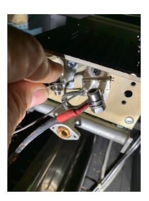
13. Reattach the gas line using Leak Lock or a good sealing compound on threaded connection and do not over tighten or you could break gas line or connectors
