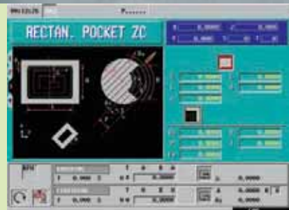
Rectangular and circular pockets associated with the C axis
