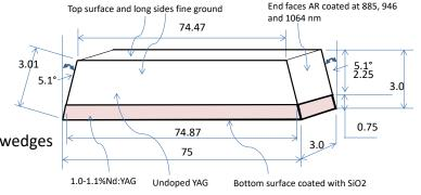
COATING Both wedged end faces AR coated at 885 nm , 946 and 1064 nm, 5.1° AOI Bottom surface coated with 1-3  $\mu$ m layer of SiO2.
