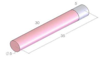
**COATING** Undoped YAG: R>99.9% @ 1064nm, Tav>97% @ 790-820nm, AOI = 0-50º Nd:YAG: R<0.15% @ 1064nm, Tav<3.0% @ 790-820nm, AOI = 0-15º Page | 15
