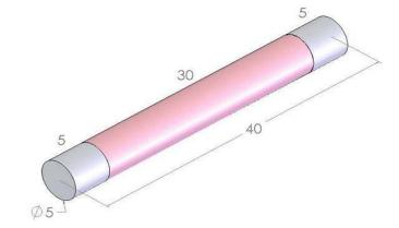
**COATING** Undoped YAG: R>99.9% @ 1064nm, Tav>97% @ 790-820nm, AOI = 0-50º Nd:YAG: R<0.15% @ 1064nm, Tav<3.0% @ 790-820nm, AOI = 0-15º
