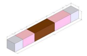
COATING One end: T>95% @ 808nm, T>95% @ 885nm, R>99.9% @ 1064nm
