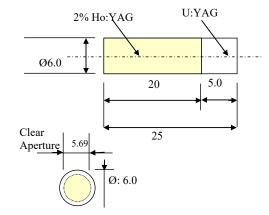
**COATING** AR/AR between 1905nm-2096nm with R<0.5% at 1905 And 0.25% at 2090nm
