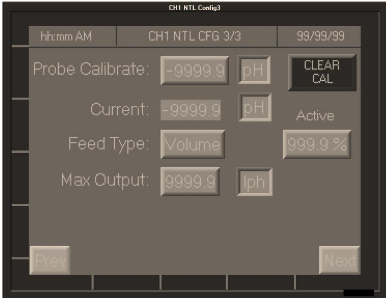
Figure 17: NTL Mode Configuration Screen 3 (of 3)
