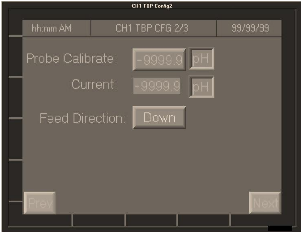
Figure 11: TBP Configuration Screen 2 (of 3)
