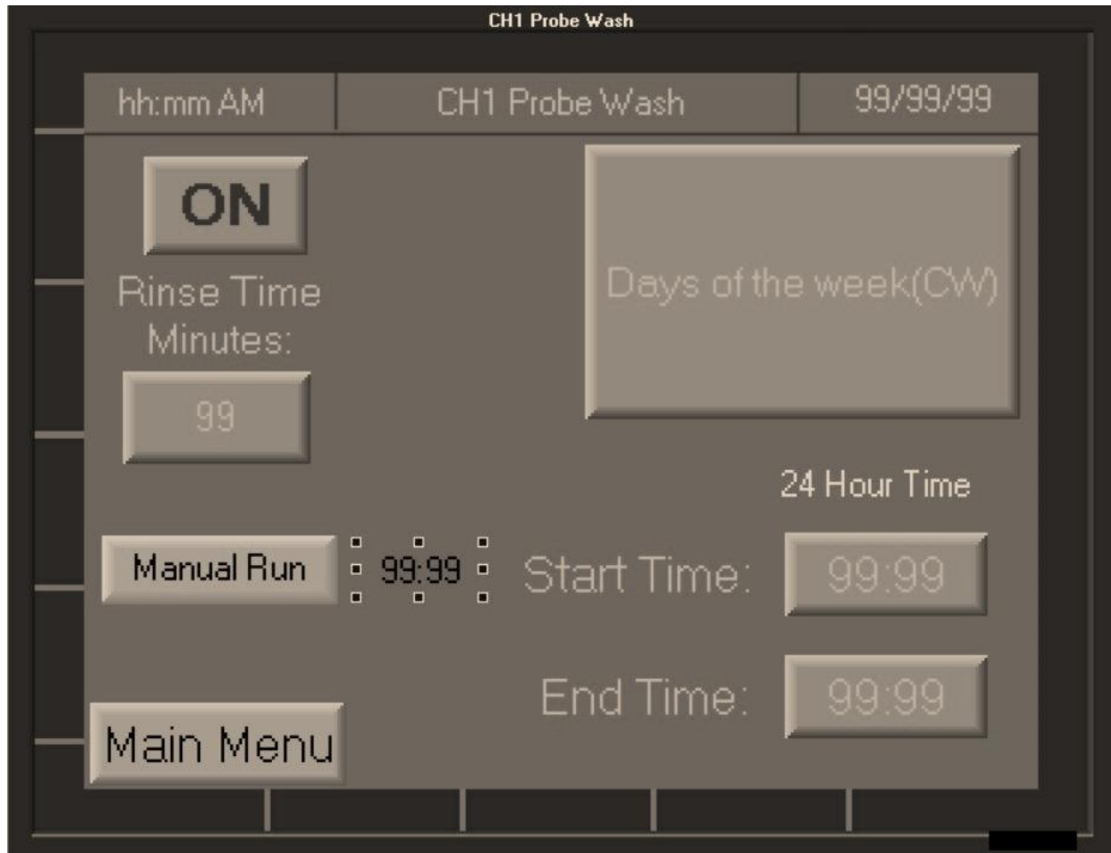
Figure 31: Probe Wash Settings Screen
