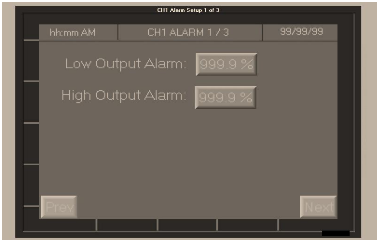
Figure 18: NTL Alarm Setup Screen 1 (of 3) – Feeder Output Alarm Settings
