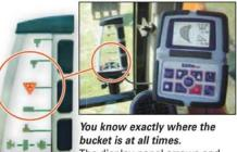
The display panel arrows and LCD direct you to the desired depth and slope.
