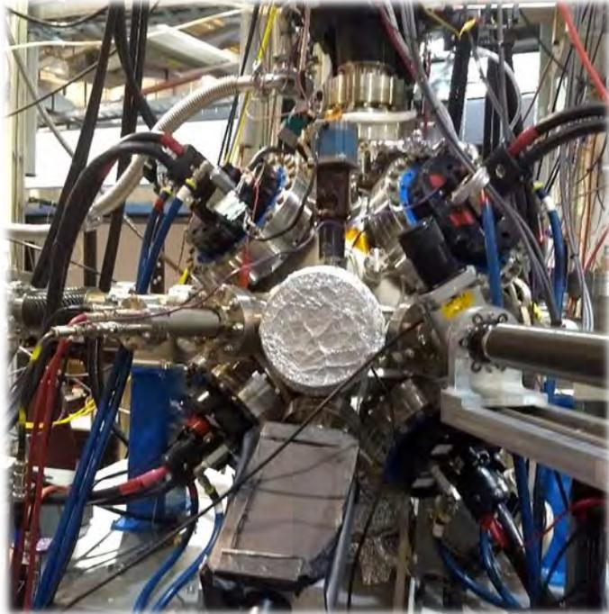
**Figure 4:** Octupole on APS beamline
