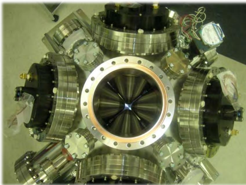
**Figure 1:** Looking Into the Octupole
