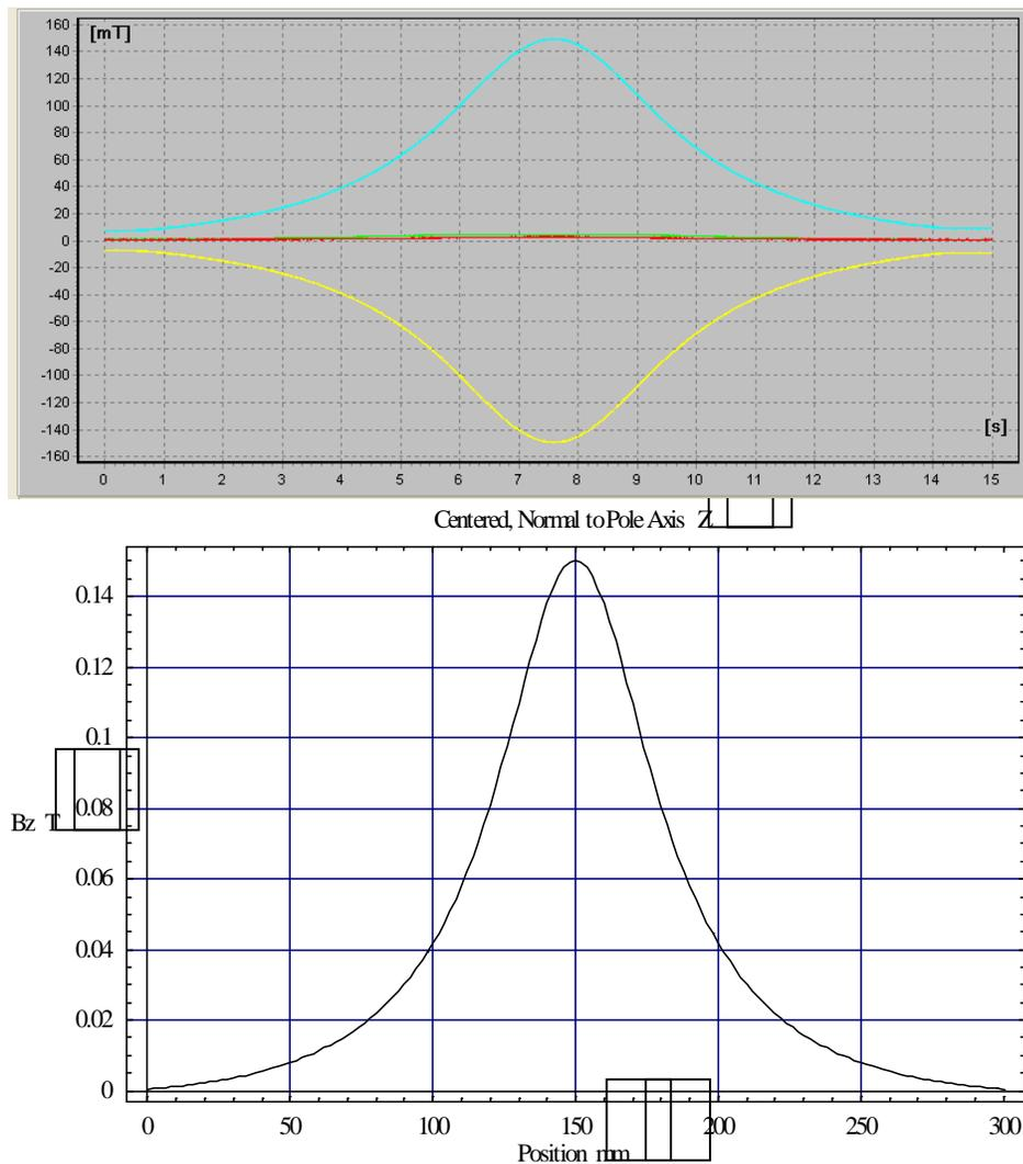
**Figure 3:** Top, dipole test results at 25 A running perpendicularly through pole center; note the x-axis is travel time
