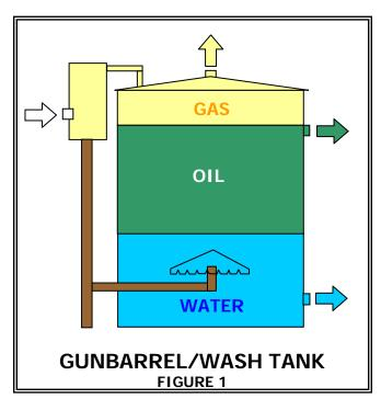
For well over 100 years the oil producing industry has used a design which is known as the wash tank, or gun barrel to dehydrate crude oil. In this design the focus is on removing water and BS&W from produced crude oil, with no emphasis on water quality whatsoever.
