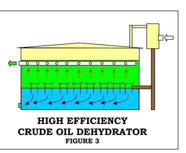
and emulsion through the entire cross section increased retention times by a factor of 10 to 35.
