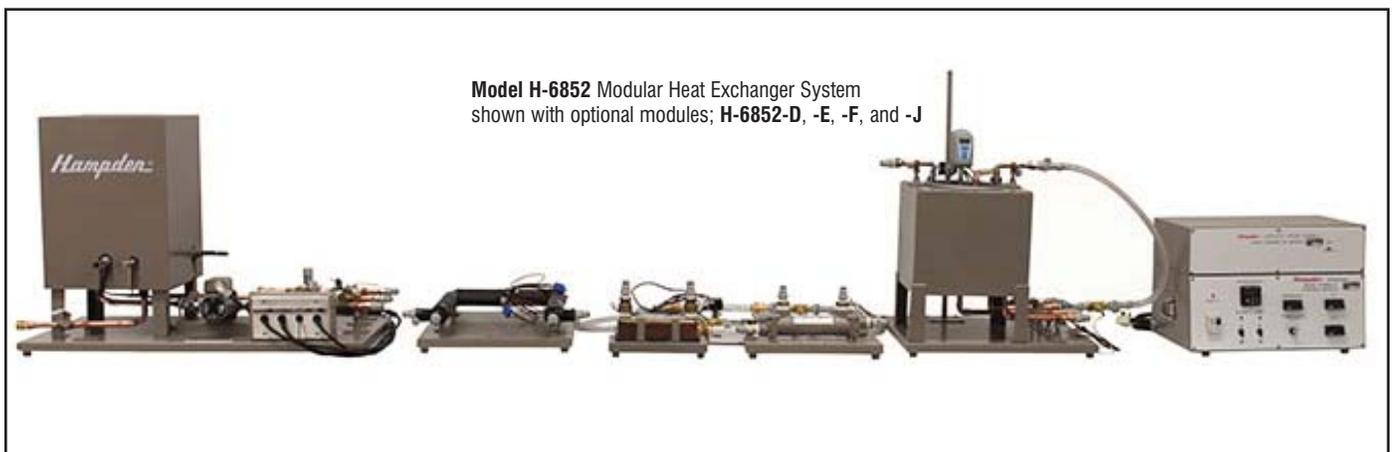
**Model H-6852** Modular Heat Exchanger System shown with optional modules; **H-6852-D**, **-E**, **-F**, and **-J**
