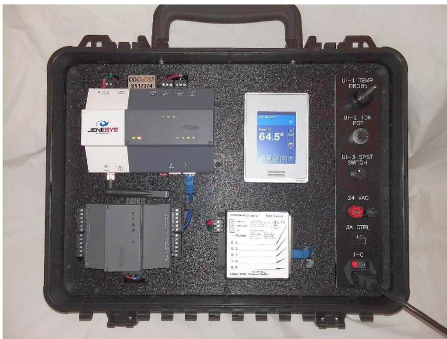
simulation of live inputs. The PT-8000s can be operated stand alone or easily networked together for use in a learning center environment. A “Startup Demo” station allows for initial orientation to the PT-816. The Demo station can be modified or replaced to meet the requirements of the specific instruction
