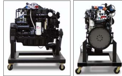
Hampden's series of full size cutaway engines provide a complete training experience. Interior components are color coded.
