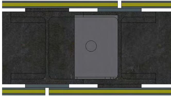
FIGURE 7: Joint between two straight wall segments.
