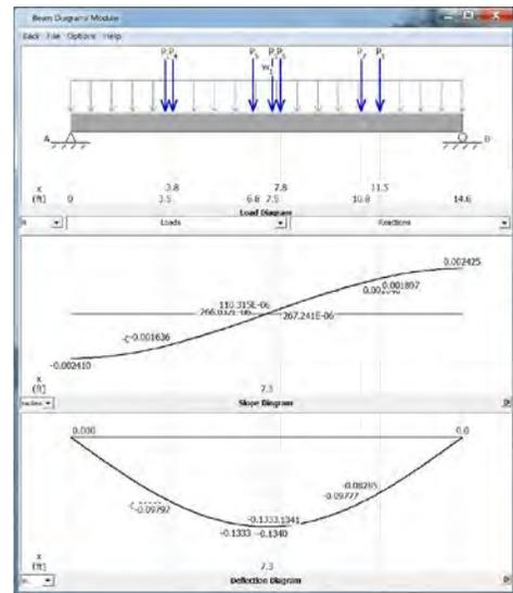
FIGURE 3: Example of calculations used in the framework design.
