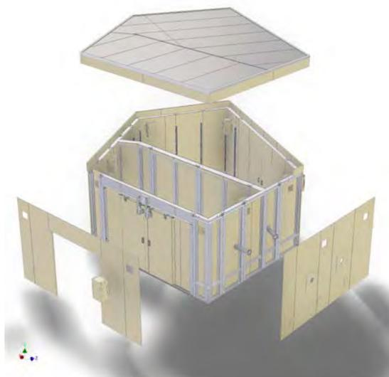
FIGURE 1: Two adjoining hutches with ceiling and exterior lead panels moved to show interior detail.
