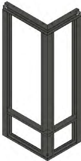
FIGURE 2: An example of a frame module, a 90° corner.
