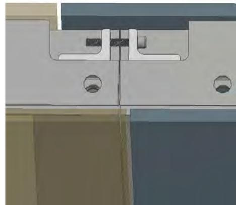
FIGURE 5: Top of wall connection.
