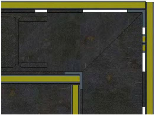
FIGURE 6: Lead detail in a corner segment.
