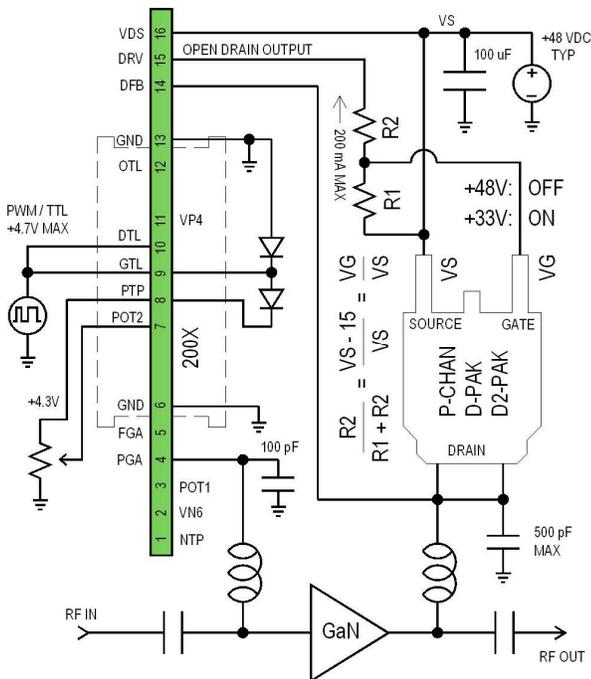
The diagram above shows a controller with an open-drain output driving a CW switch. It can be seen that the gate voltage to the MOS device is always 15V below the source level to turn-ON the switch. Therefore,
