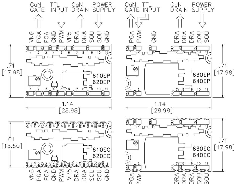
TYPE-EP typically mounts on metal surfaces, while TYPE-EC on printed circuit boards.
