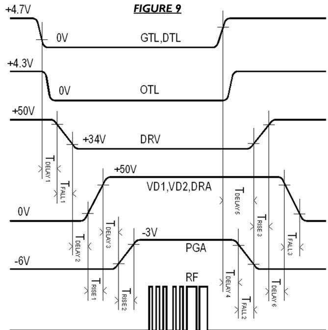
Only with the presence of drain voltage would the gate switching feature activate (PGA), and finally turns on the GaN device for RF to transmit. The sequence is finished with the rising end of the TTL signal. The pulsed gate (PGA) goes back to pinch-off voltage and drain voltage (VD1, VD2, DR) shuts down thereafter. Note that the total ON propagation time from TTL to RF is the sum of time delays, rise times, and fall times shown in the diagram. Total propagation times of <500nsec are common.
