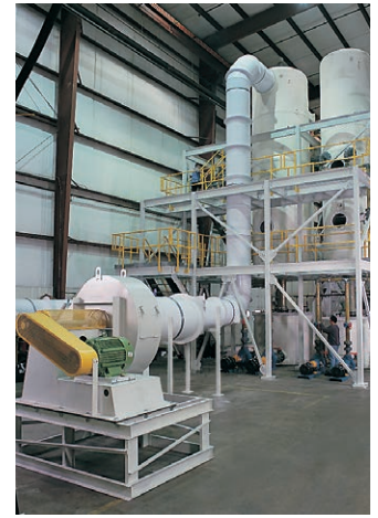
Fiberglass-constructed, 2-stage HCl scrubber with dual fans and catwalk assembly.
