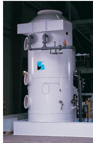
Single stage V/F series packed scrubber with dual pumps and containment pan constructed of UV-stabilized polypropylene.
