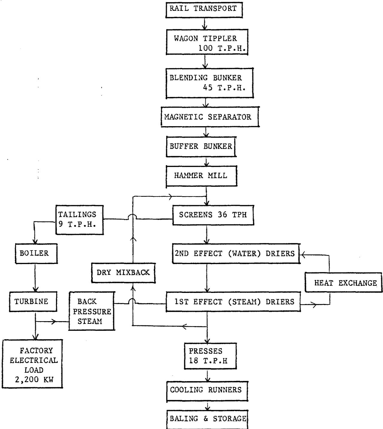
Fig. 5.1 - Irish Briquette Factory Flow Diagram
