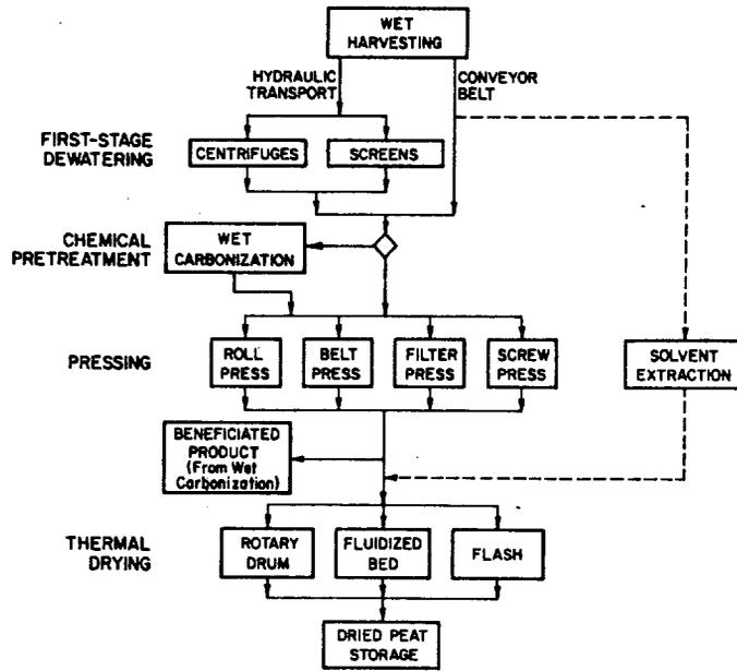
Fig. 5.2 - Alternative Dewatering Methods of Peat
