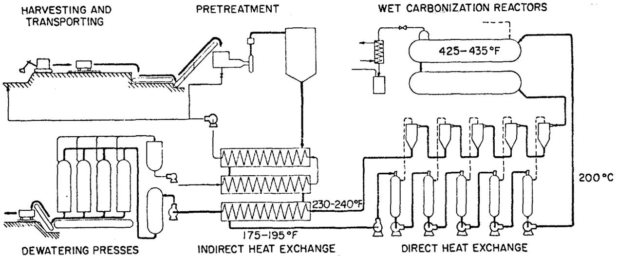
**Figure. 5.4 - Swedish Wet-Carbonization Process Flow Diagram**
