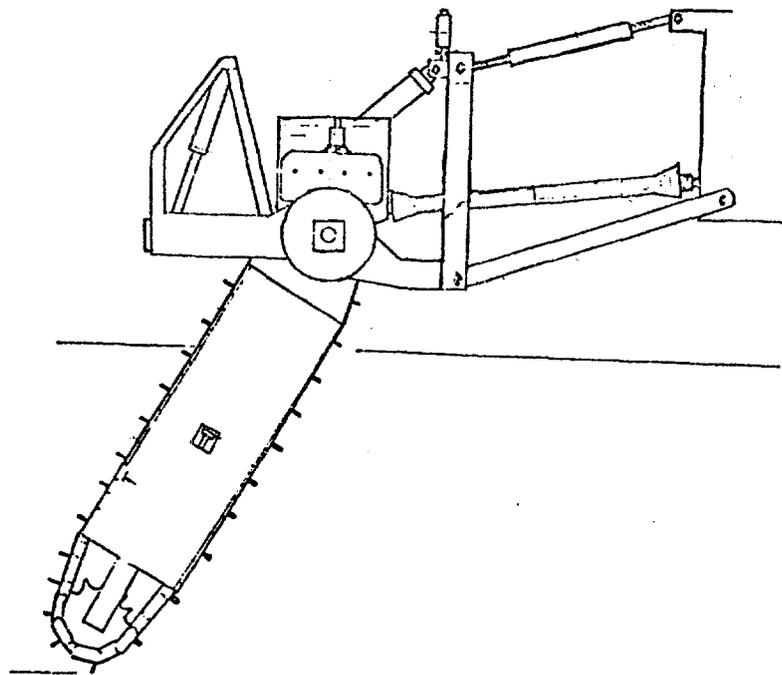
Fig. 4.4 - Chainsaw Type Sod Peat Production Machine
