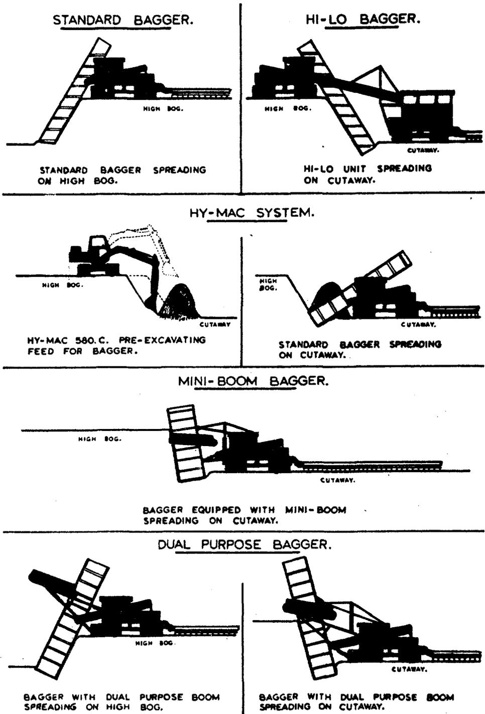
Fig. 4.2 - Bagger Systems of Sod Peat Production
