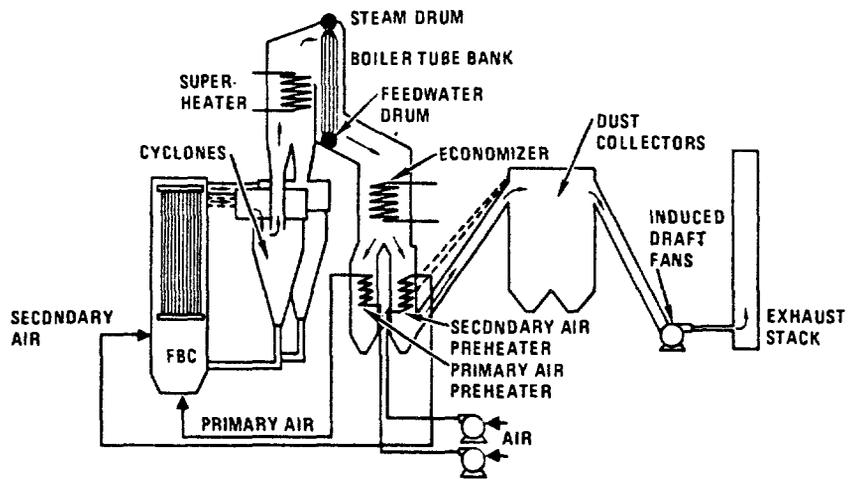
Fig. 6.4 - Schematic Layout of a Fluidized Bed Boiler
