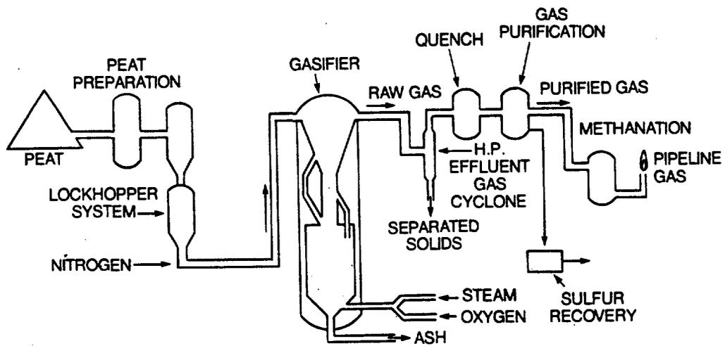
Fig. 5.6 - PEATGAS Process Flow Diagram
