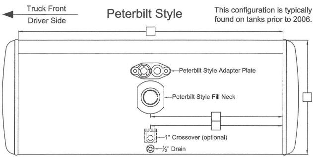
Please note: All sizes are NPTF unless otherwise noted and reference all measurements from the lateral weld seam and the end cap weld seam to the center of the fittings.
