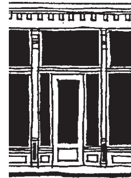
Original storefront doors were typically recessed, constructed of wood with a large window above a single or double panel that complemented the bulkhead design below the display windows
