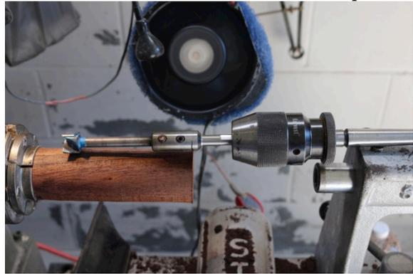
Mix up some 5-minute epoxy and coat the inside of the hole and outside of the coupling, use the lathe to push the wood onto the PVC coupling. I have found that some Teflon tape keeps me from gluing the PVC coupling to the brass nipple! The "V" grooves act as keys to keep the coupling in place.
