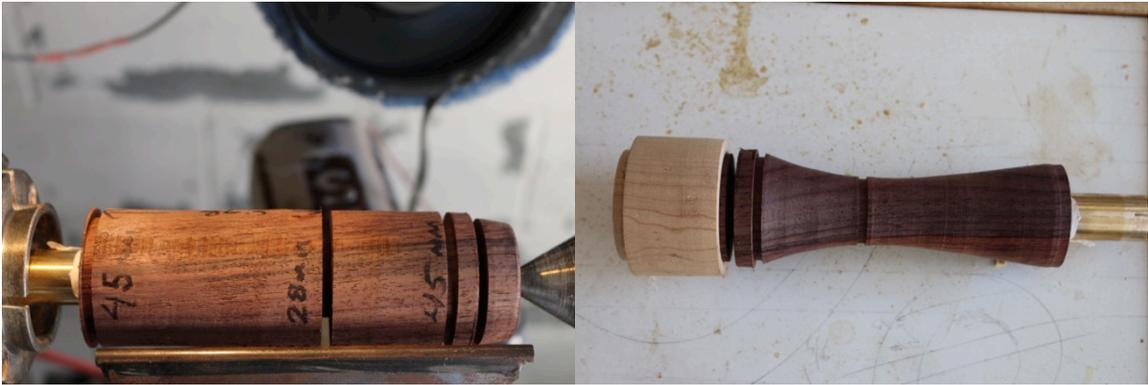
I have made a drilling jig that requires that I turn a taper on the waste area above the top, where the old tendon was originally cut. This takes a little time to get just right but lets me drill the holes quickly.
