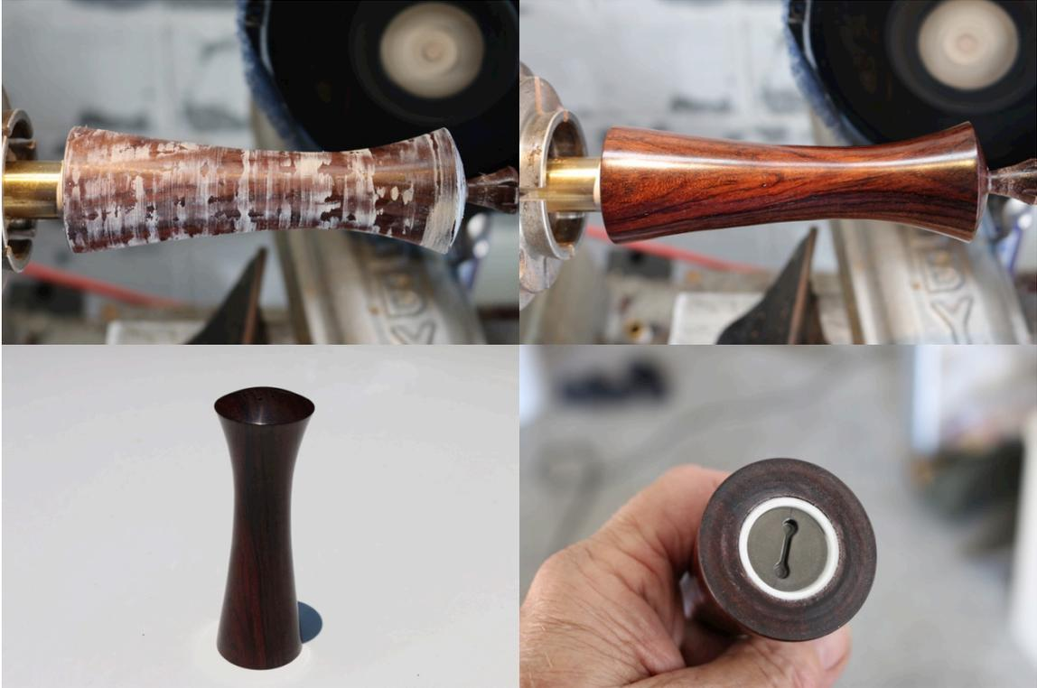
Finish by cutting the nib from the top and sand to 320-grit, dab a little lacquer on the fresh wood and finish with HUT wax.
