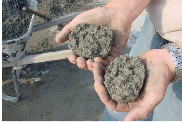
Very Low Slump Concrete
