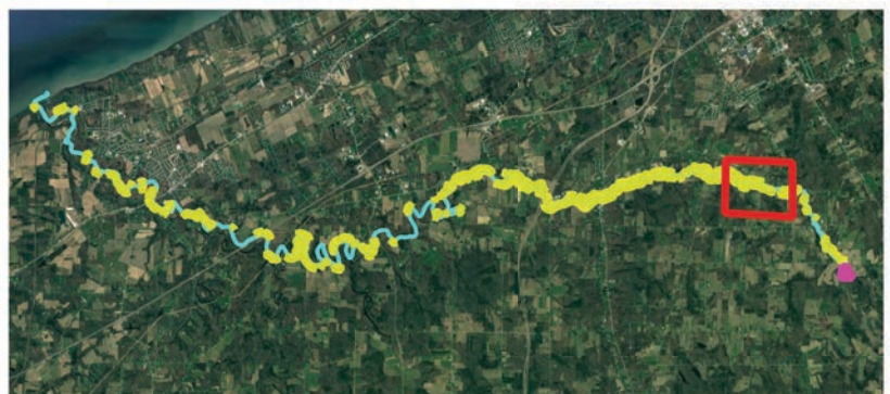
Exhibit 19. Example of upland areas within 300 ft of Elk Creek interspersed with NWI mapped wetlands. Right, overview of Elk Creek drainage. The red square indicates the area zoomed above.
