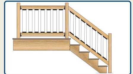
**STEP #6** - Install stair rail assembly.
