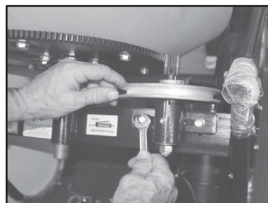
Step 7 Slide drum on frame. Then install pinion housing. Line up front of pinion with front large gear (Note: Do not position pinion to far forward, so gear will dig into drum.)
