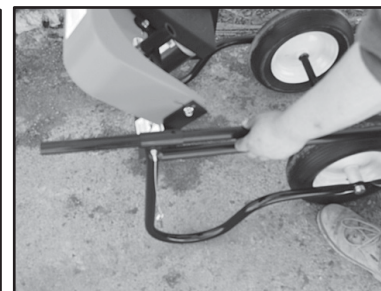
Step 11 Slide handle in place lining up the hole in the handle and the housing. Slide the pin through the holes.
