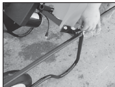
Step 12 Slide the pin through the holes. Soak Grips in boiling water for 1 minute to soften the heavy duty rubber.
