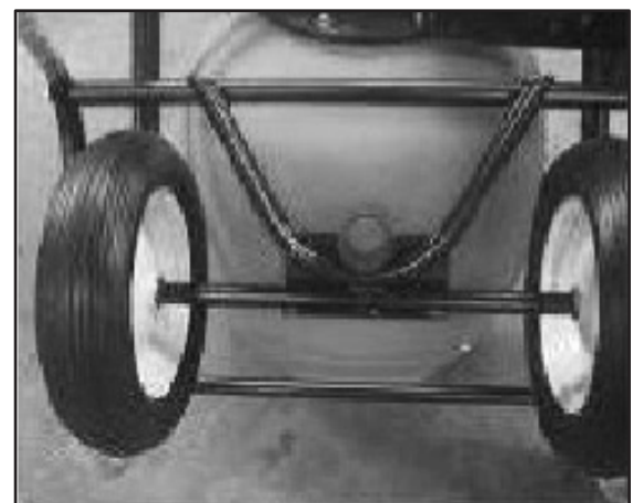
Figure 7 – Rotate Pivot Mount Plate to wheelbarrow stowed position
