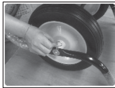
Step 4 Put washers on the axle, then fix R clips into holes.
