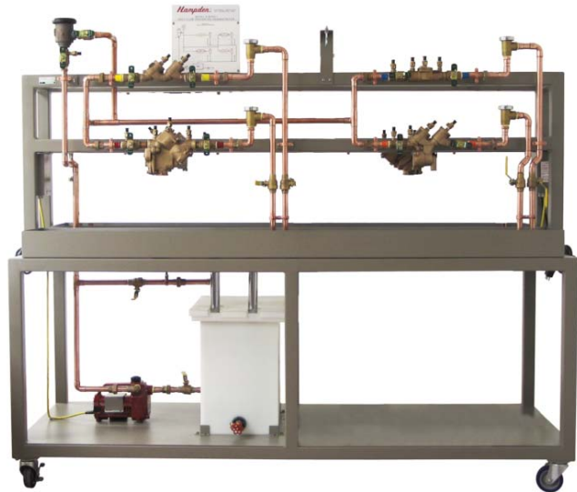
H-BFPD-2 Single Sided Back Flow Prevention Demonstrator
