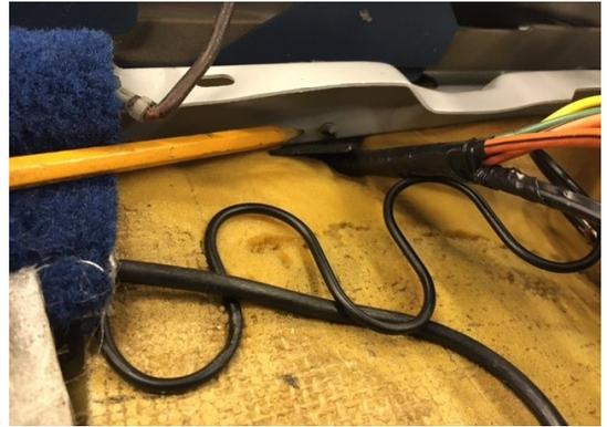
**ly** found. There is a place in the harness for the seat switch where 2 power wires are soldered to one, and the insulation had come apart there, hitting the seat frame. I rewrapped it, and placed some thin rubber between it and the frame, and hopefully that is fixed once and for all!
