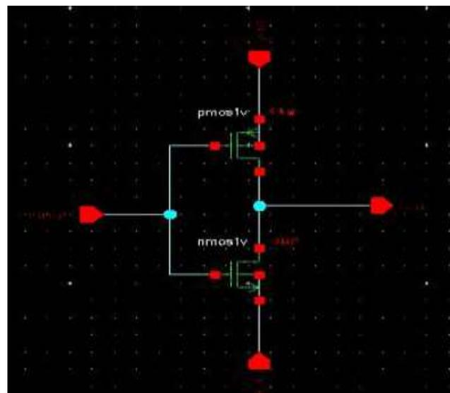
Fig. 1. Schematic of an Inverter
