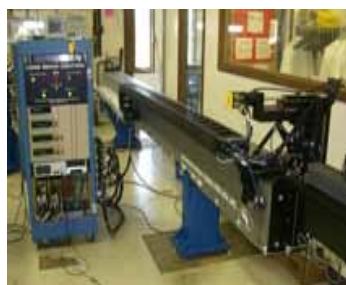
SSRF Magnetic Field Measurement System
