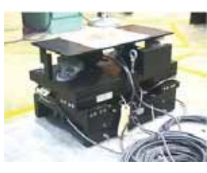
Compact Precision Translator for LANL Neutron Facility
