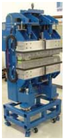
Synchrotron Radiation Center (SRC) Planar Undulator
