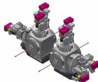
Custom Monochromatic UHV Slits BL02B at SSRF
