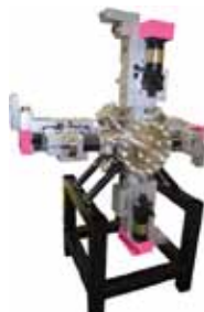
UHV Slit System for ESRF
