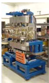
BNL Cryo In-Vacuum Undulator
