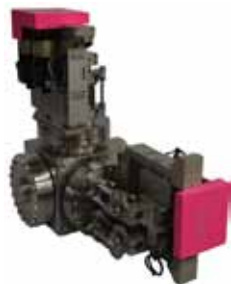
SwissFEL High Precision Slits (Curtain Design)
