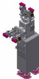
LSU/CAMD Water Cooled UHV Slits
