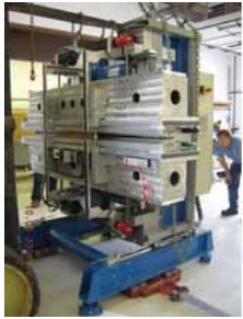
MAX Lab Hybrid EPU Undulator
