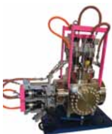
High Heat Load UHV Slit System for ESRF ID11 Pinhole Mono
