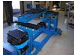
Four-Axis Goniometer for the Canadian Neutron Beam Centre
