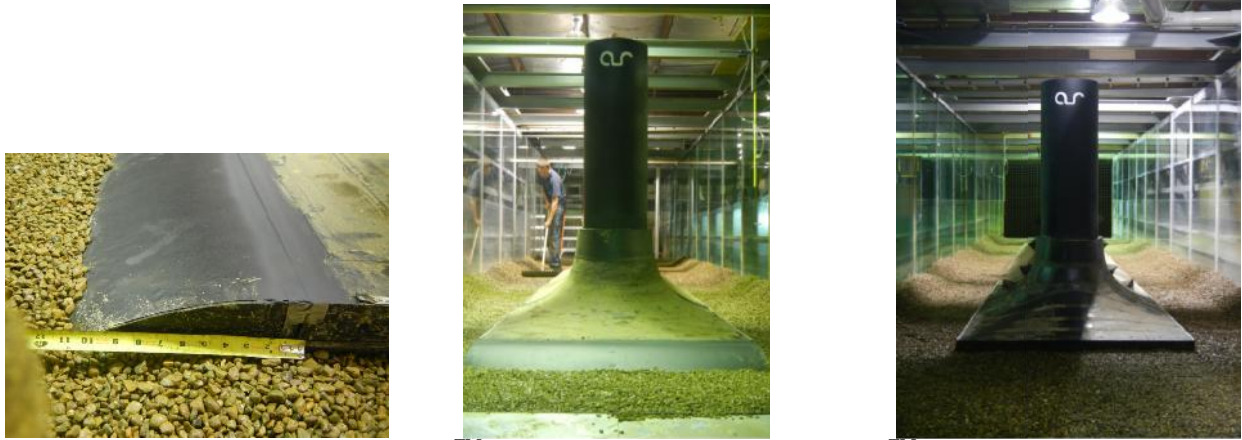
Figure VII.7 Configuration C: sCAUR™ full-scale model with 8 VorGAUR™ VGs raised 3" above gravel bed with leading edge ramp (left). Looking downstream (middle photo) and looking upstream (right photo).
