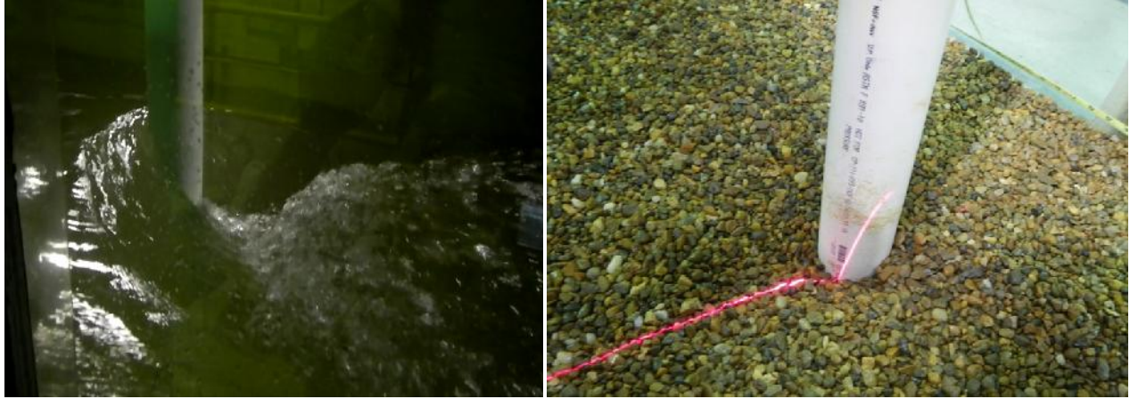
Figure VII.5. Surface bow wave around the 3.5" (88.9mm) diameter comparison circular cylinder during a test (left). Equilibrium large-sized gravel scour hole in front of 3.5" (88.9mm) diameter circular cylinder and laser sheet (right); typical for tests for all Configurations.
