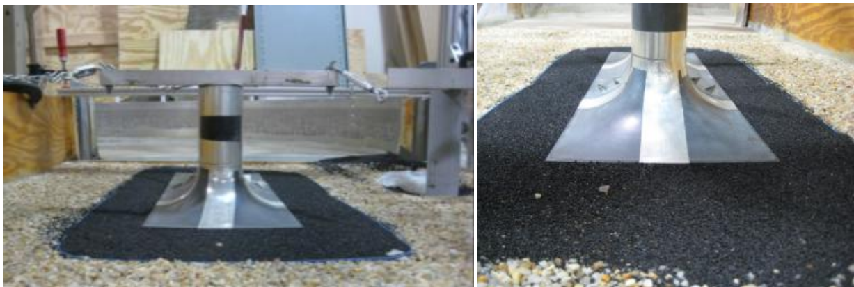
Figure III.3. Black slag gravel A around sCAUR™ model showing no scour after a test. View from upstream (left); view from downstream (right).
