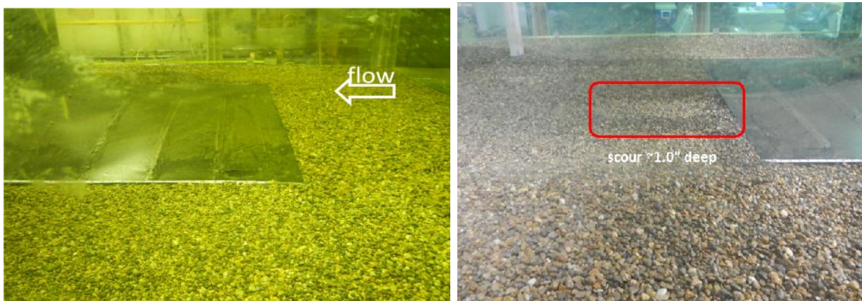
Figure VII.4. Configuration A: no scour of small or large gravel around front and sides of full-scale scAUR™ model with 6 VorGAUR™ (left); scour of smaller gravel downstream of model (right). Flow from right to left.
