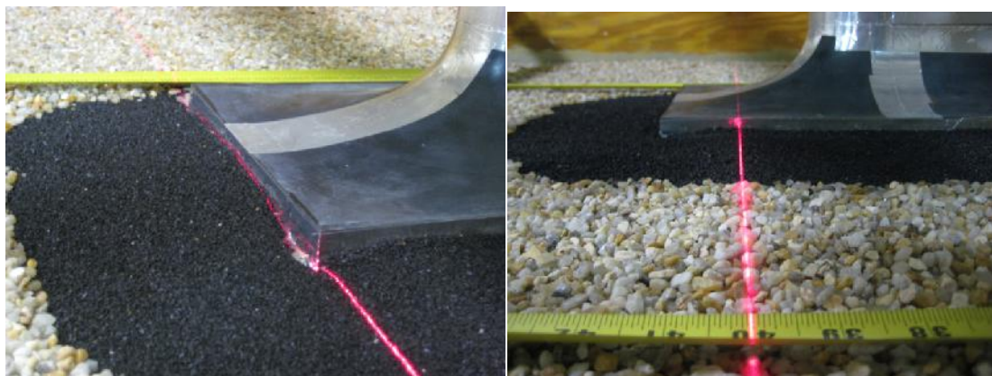
Figure V.3. Gravel level after flume test for 0.5" (12.7mm) high elevation without a leading edge ramp . Note laser sheet for gravel surface measurement. Note scour at the front corners of the foundation.
