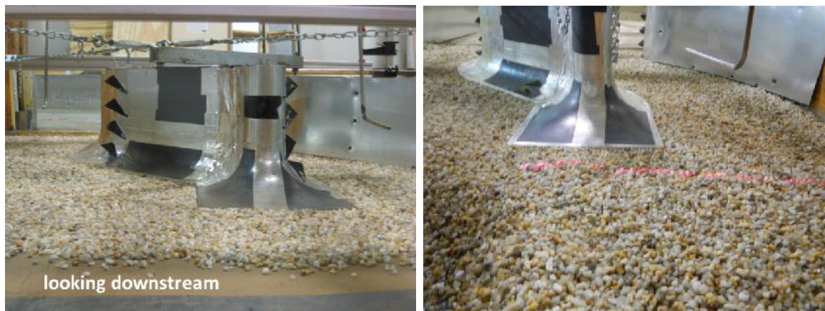
Figure IX.2. Photos of pier nose and stern additions to the AUR model used in AUR flume tests. (left) Upstream view showing location of VGs on model front right and rear left sides. (right) Laser sheet showing no scour downstream of the model.
