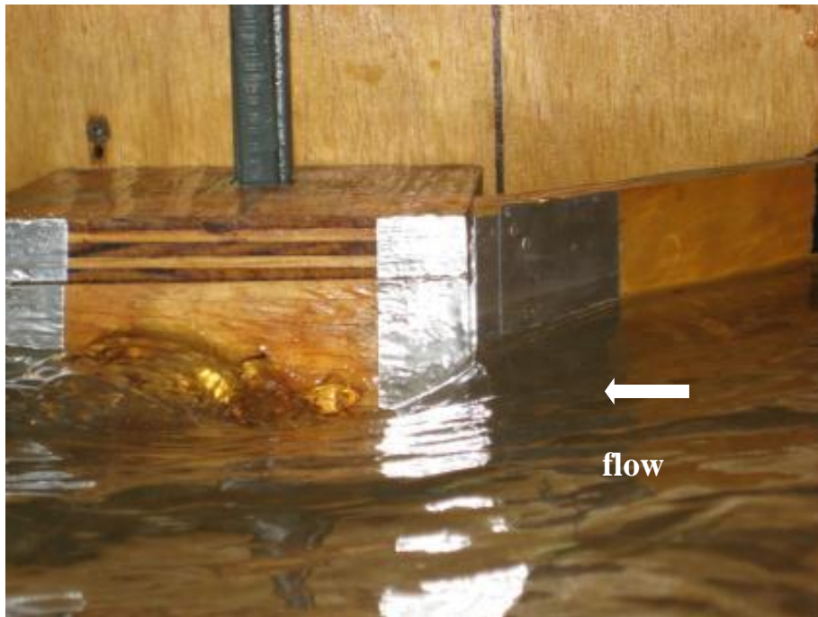
Figure IV.2. Closeup view of wing-wall abutment model. Note that free surface height change after the leading edge of the contraction due to separation.
