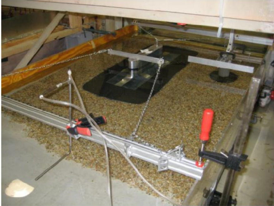
Figure III.1. Photo of AUR 4 foot (1.22m) wide flume test section looking downstream with black gravel around the scAUR™ model (middle of photo), the comparison circular cylinder (right of photo), and pea gravel away from the model. The 1/8" to 1/4" (3.18mm to 6.35mm) pea gravel produces open bed scour at higher water speeds than the open bed scour of the black gravel. Note the location of the pitot-static probe 1m upstream of the scAUR™ with VorGAUR™ model.
