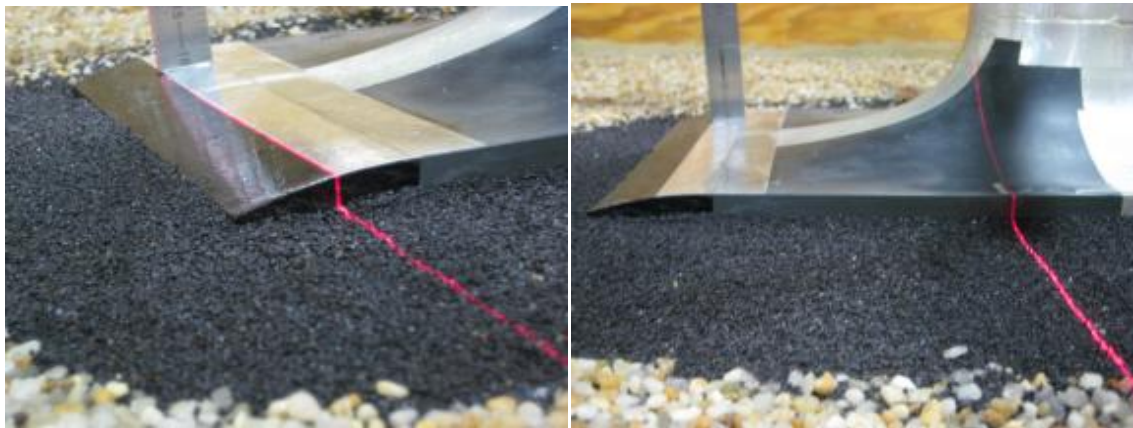
Figure V.5. Gravel level after flume test for 0.5'' (12.7mm) high elevation with a 0.75'' (19mm) high curved-top rectangular planform straight-sided leading edge ramp buried 0.25'' (6.35mm) in the gravel. Note very little scour around the foundation.
