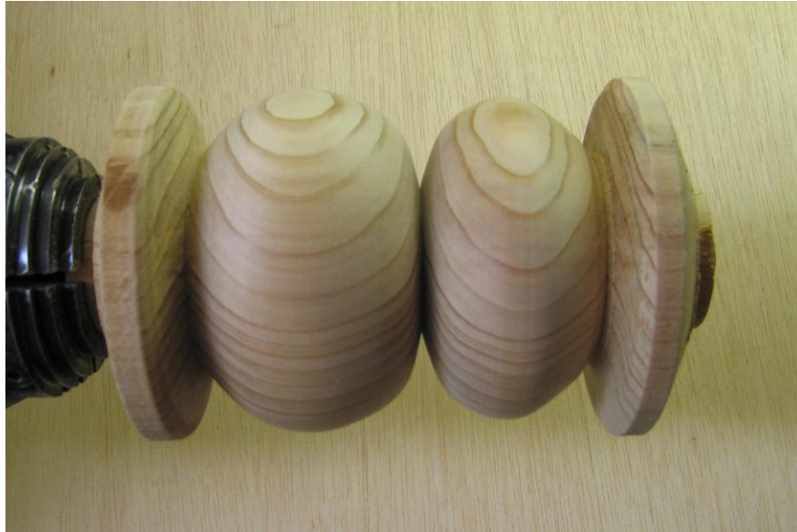
Finished box on first axis
