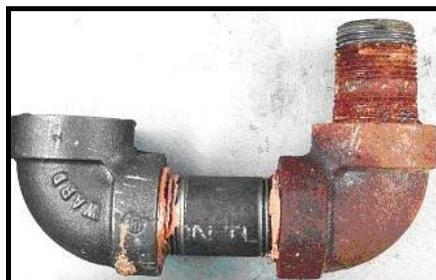
**Figure 6– Stainless Steel Corrosion**
