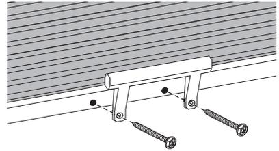
**CAUTION:** To prevent damage to the shade do not overtighten the screws.
