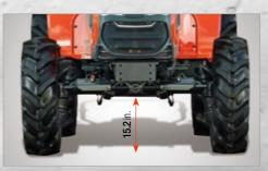
High Ground Clearance The maximum ground clearance of 15.2 in. makes usage on rocky or uneven terrain simpler.
