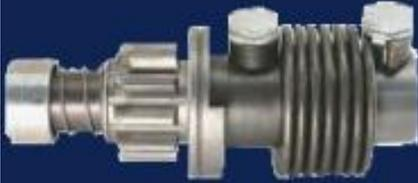
The small Bendix Drive gear that's bolted to the starter motor puts up with a lot of use (and abuse when you forget to retard the spark before starting). Eventually you will be working on yours and I have a tip for you about installing it back on the starter shaft.
