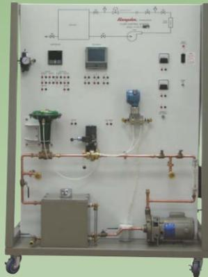
The **Model H-ICS-FX** Flow Control Trainer is designed to provide complete instruction on the measurement and control of flow of energy. The rate of water flow is dependent on the position of the control valve and on the position of a hand-operated valve. ◀◀◀◀
