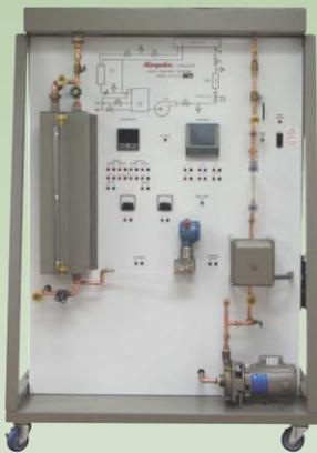
The **Model H-ICS-LX** Level Control Trainer is designed to provide complete instruction on the measurement and control of level. Tank level water flow is dependent on the position of the control valve and the rate at which water is allowed to flow (by gravity) into the tank. ◀◀◀◀
