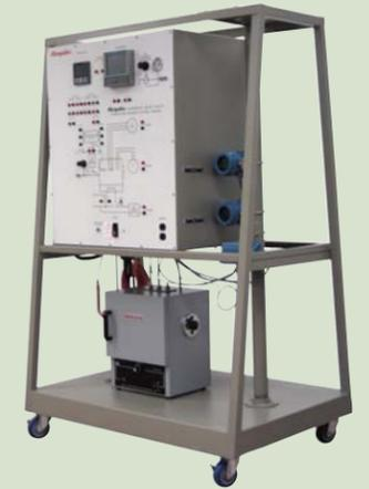
▲ The **Model H-ICS-TT** Temperature Process Loop Trainer is designed to provide complete instruction on the measurement and control of temperature.
