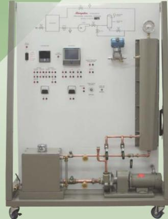
The **Model H-ICS-PX** Pressure Control Trainer is designed to provide complete instruction on the measurement and control of pressure. Pressure within the vessel is dependent on the speed of the pump and the open or closed position of hand valves that permit flowing water to bypass the pressure vessel. ▶▶▶▶
