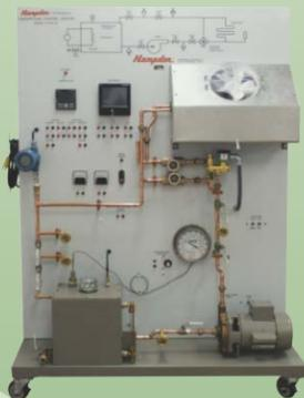
The **Model H-ICS-TX** Temperature Control Trainer is designed to provide complete instruction on the measurement and control of temperature. The temperature is dependent on the current through the heater and on the position of the solenoid-operated three-way valve. ▶▶▶▶
