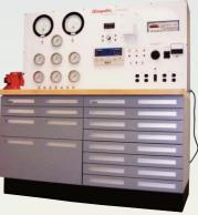
**Hampden H-9067** Instrumentation Test Bench provides a complete platform for instrument calibration.
