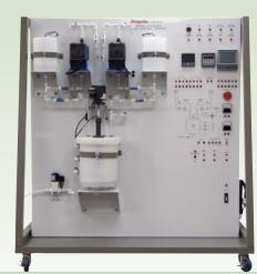
The **Model H-ICS-X** Instrument and Control Interface Package and Program consists of the hardware and software necessary to control the Hampden series of ICS panels. This is a graphically-oriented program, with documentation, to permit computer control of the panel's controller.
