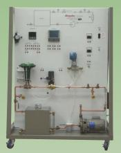
The **Model H-ICS-FX** Flow Control Trainer is designed to provide complete instruction on the measurement and control of flow of energy. The rate of water flow is dependent on the position of the control valve and on the position of a hand-operated valve.
