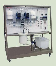
The **Model H-ICS-HET** Heat Exchanger Process Loop Trainer is designed to provide instruction on the measurement and control of temperature utilizing a heat exchanger or a SCR. Temperature
