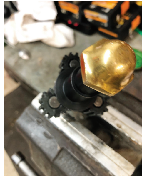
3) Steering wheel nut on pinion post for using a socket wrench
