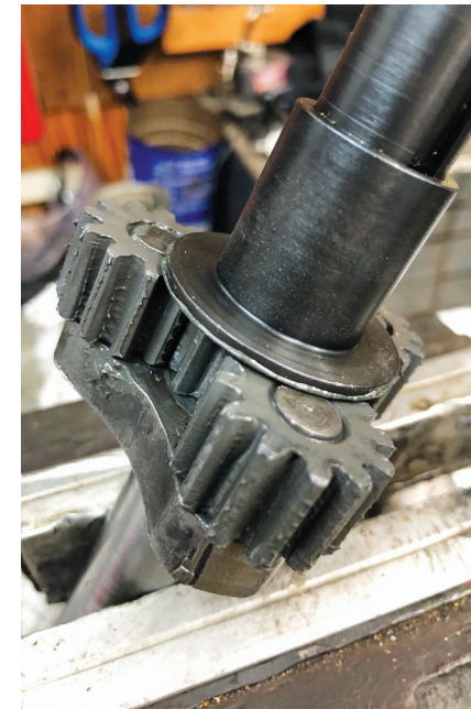
5) Smooth gear mesh obtained by lapping
