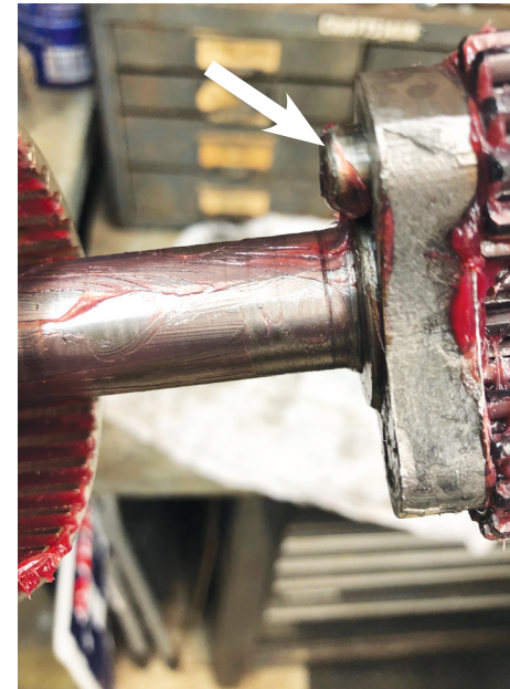
7) The longer pin fits into the groove of the steering case
