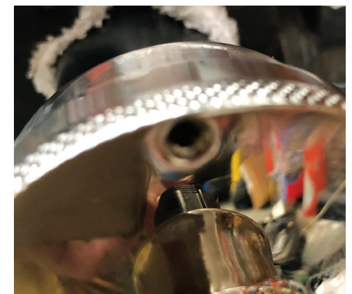
10) Align the holes in the steering case and cover for the important retaining screw
