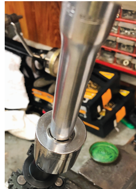
4) Socket wrench used to turn gears
