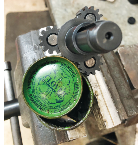
1) Valve grinding compound is useful for lapping the steel gears
