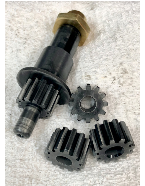
6) Lapped and cleaned gears with drive pinion, showing the burnished teeth. Ready to install.
