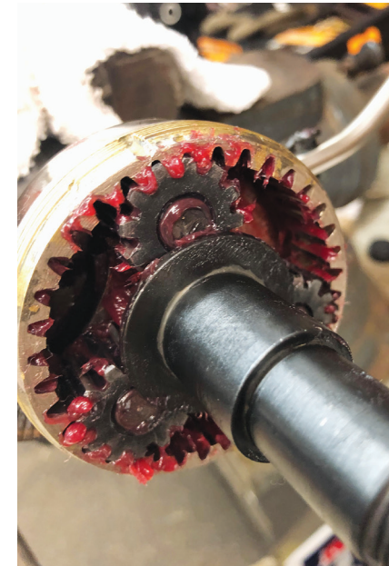
8) Greased gears and drive pinion installed
