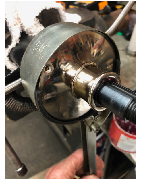
9) An oil filter strap wrench helps tighten the steering case cover
