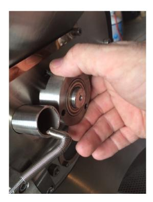
If bearing holder is hard to remove you may use its own screws placed into bearing holder against front plate (away from existing screw holes) And screw into holder to push the bearing and its holder out off shaft. (See picture below)- You can also use bearing pullers if you like
