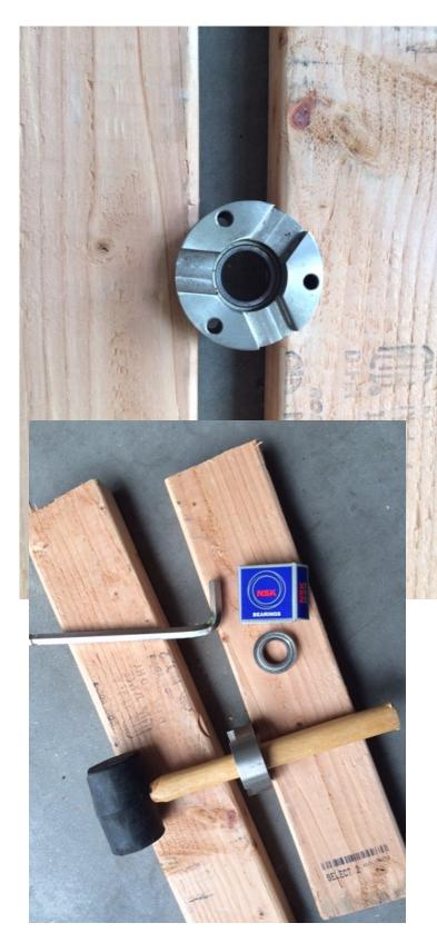
Put upside down between 2 2x4's and using a wooden dowel or handle tap bearing off holder
