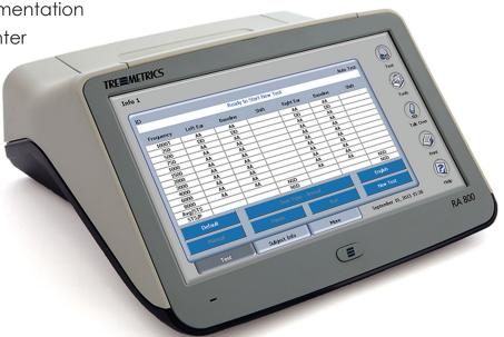
The RA 800 is the new easy-touch testing audiometer designed and built by Tremetrics, the leading manufacturer of occupational hearing testing equipment in the U.S. For over 45 years, Tremetrics has been the industry innovator – pioneering all of the major advances including microprocessor and self-recording audiometry, hearing/health database software, the OSCAR™ Electro-Acoustic Ear and interactive multi-language hearing testing capability.
