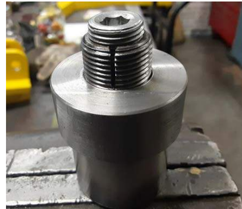
Fig. 4 Tool for Mounting Timing Cover
