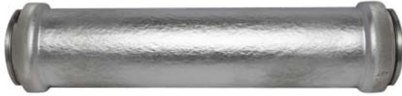
Figure 4. Fully Eroded Aluminum Target Tube implementing New Magnetic Design
