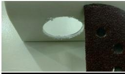
Use Sandpaper to lightly clean up edge and increase bond strength. Give it a quick wipe with acetone
