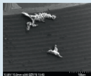
Debris left from plastic scaler
